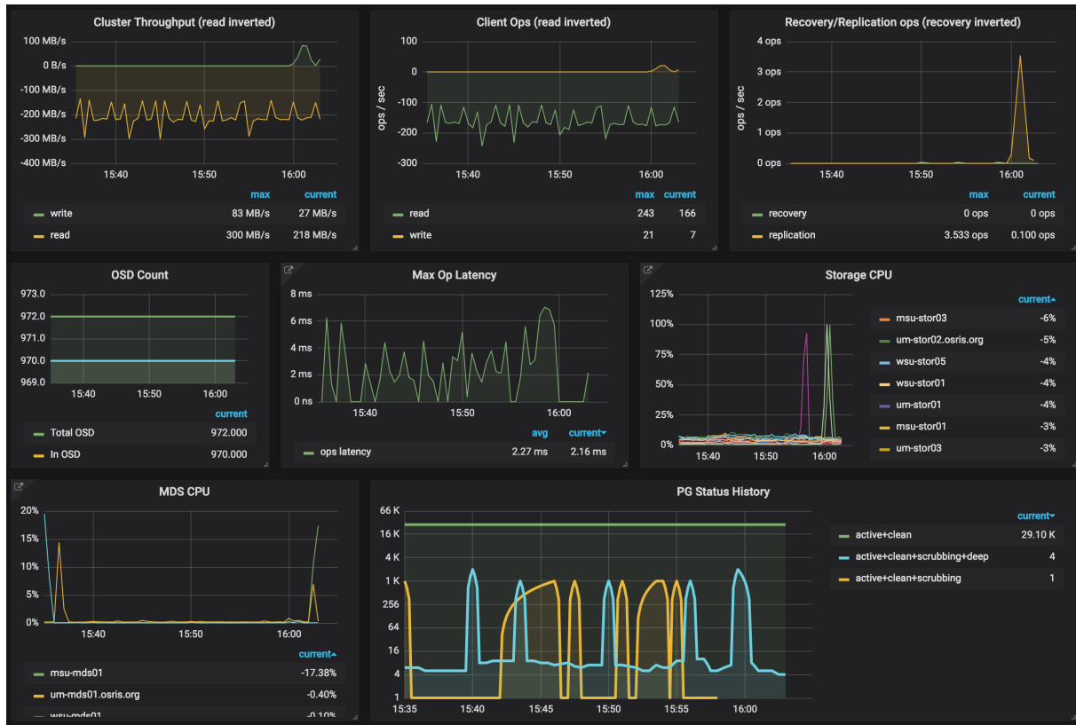
Figure 5. Example of OSiRIS Ceph cluster dashboard using stats collected by ceph-mgr InfluxDB plugin. The information presented here can tell us about cluster activity as well as cluster problems such as excessive latency, down OSD, or high load on systems
