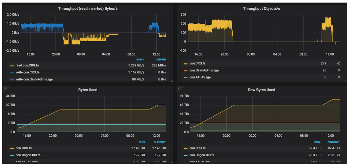
Figure 6. Example of OSiRIS Ceph cluster pool dashboard using stats collected by ceph-mgr InfluxDB plugin. The information on this dashboard tells us who is using OSiRIS at a given moment, their cumulative data usage, and whether users are getting expected performance.
