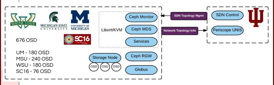
Our first site required manual steps to bring up VM host, and Foreman/Puppet installation. The rest, including Ceph components, is automated from there.
