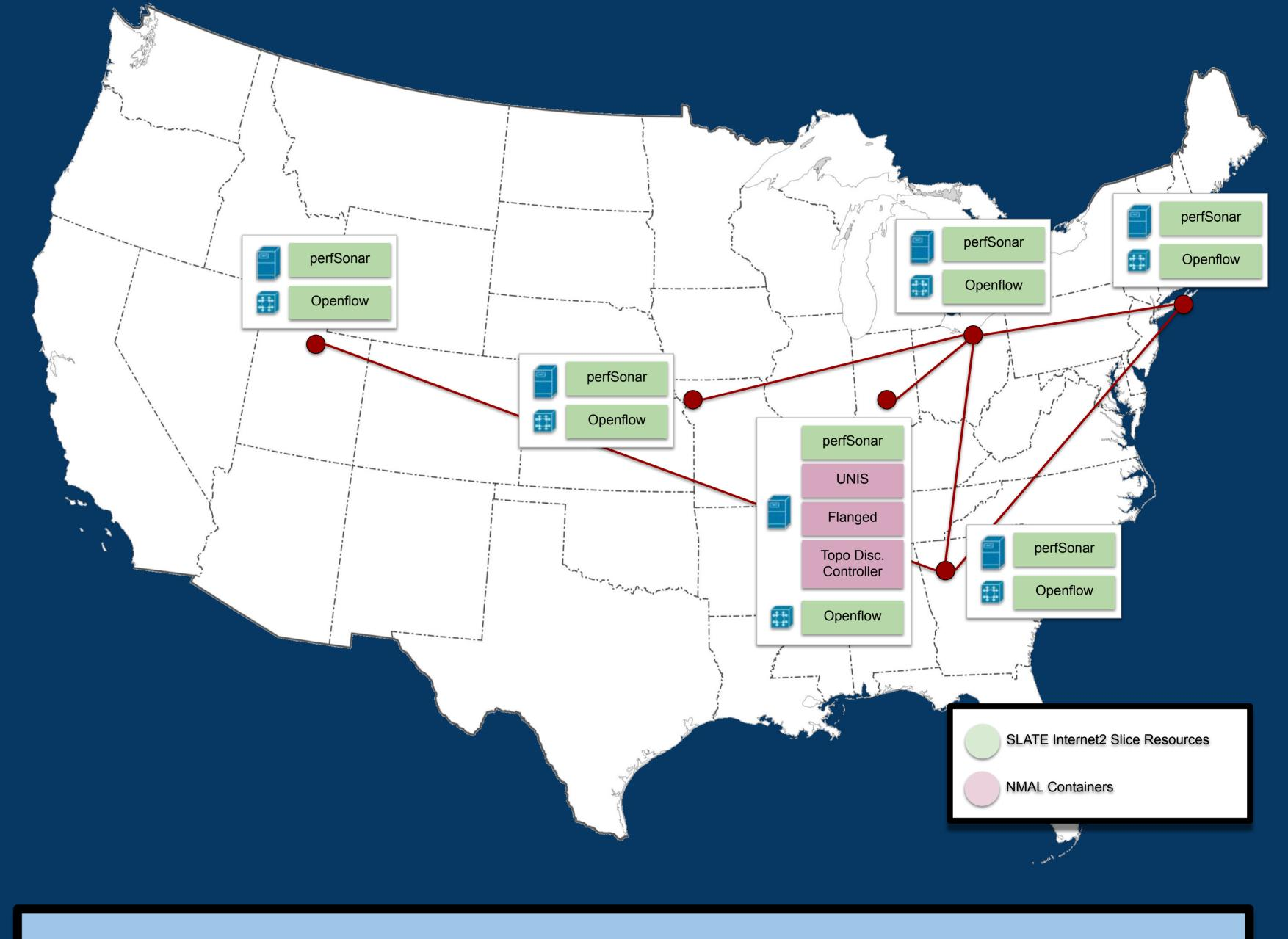
NMAL gives us real-time feedback into the topology of our network from hardware switches and software **Open vSwitches**
