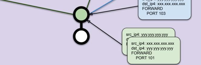
Configuration programs written in the network orchestration language, **Flange**, generate rules for a provided topology. When run against the SLATE testbed, the program above generates a single bi-directional circuit between Salt Lake City and Atlanta. This circuit is predicated on the measured performance of the underlying network. When NMAL detects a spike in bandwidth utilization, the program is partially re-evaluated and a new set of rules is generated to satisfy the program.
